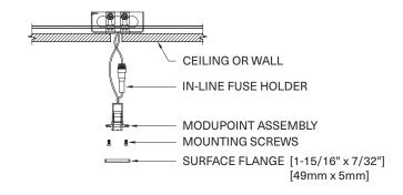
Housing: Recessed with 1-15/16" [49mm] surface flange
