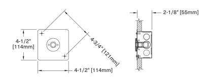
Housing: Recessed EQ Modupoint with 1-15/16" [49mm] surface flange is factory installed on plate
