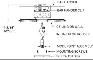
Housing: • Recessed with 3-3/8" [85mm] diameter x 1/4" [5.5mm] thick threaded surface flange
