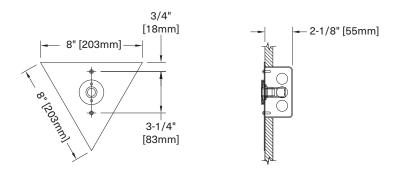
Housing: Recessed EQ Modupoint with 1-15/16" [49mm] surface flange is factory installed on plate
