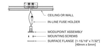
Housing: Recessed with 1-15/16" [49mm] surface flange
