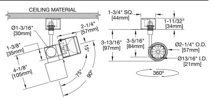
Housing: Fabricated aluminum and steel
