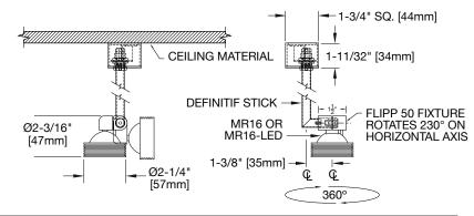
Housing: Fabricated aluminum and steel
