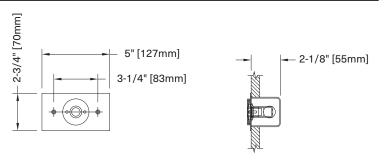
Housing: Recessed EQ Modupoint with 1-15/16" [49mm] surface flange is factory installed on plate
